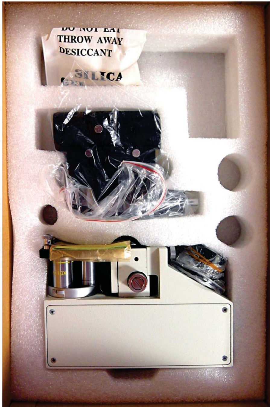
Figure 8. Current FM-31 clone with attachable illuminator, stored in original packing Styrofoam
