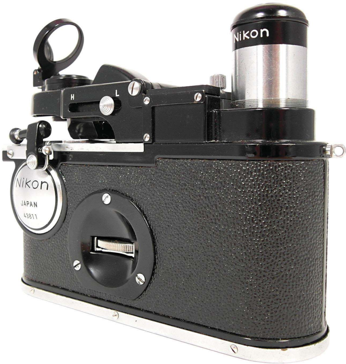
Figure 5. Nikon H folded-optics microscope, c. 1960s
